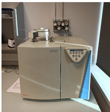
Elementinis analizatorius (Thermo Scientific Flash2000 CHNS-O)
