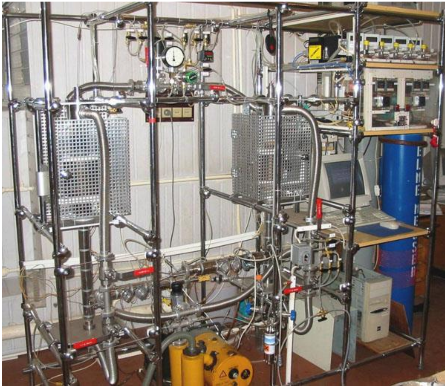
A system of two Pulsed Injection MOCVD reactors for oxide depositions
