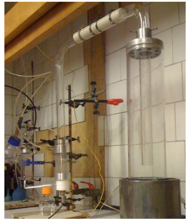
Mini aerosol –assisted atmospheric pressure MOCVD reactor (aerosol-pyrolysis reactor)
